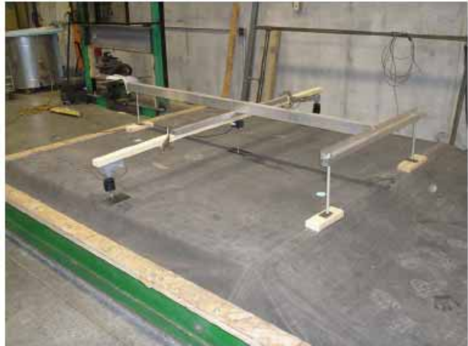
PHOTO 2: Transverse load test setup
