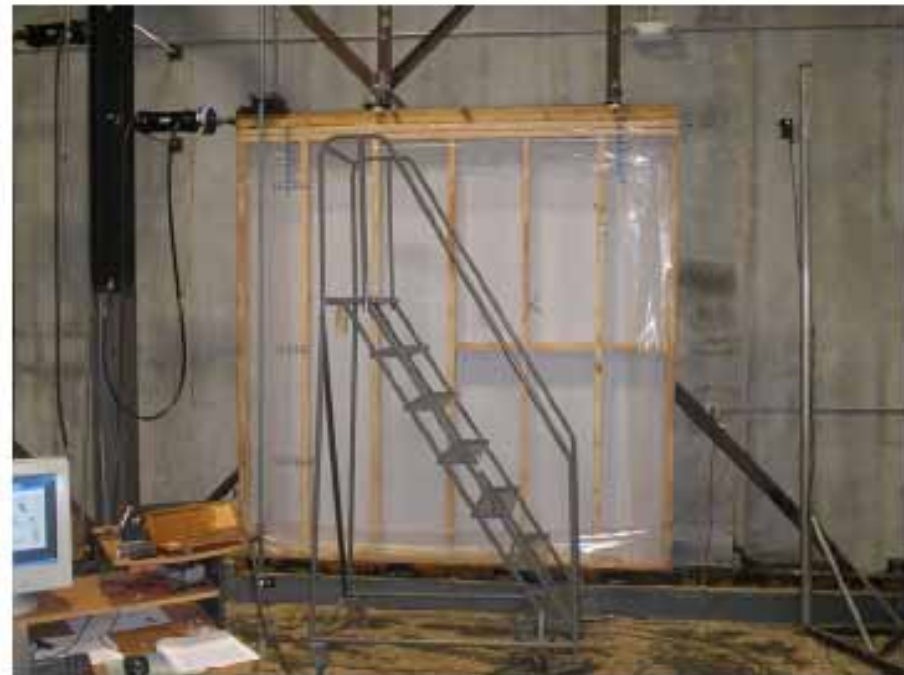
PHOTO 11: General test setup for racking load testing in accordance with ASTM E 72.
